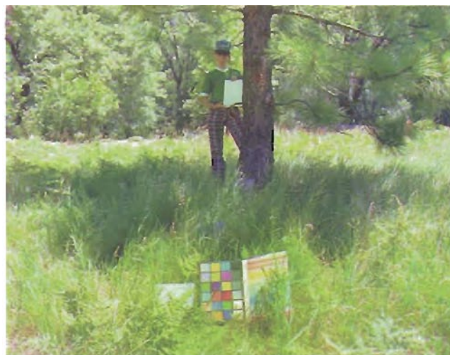
Figure 4. This is a computer-processed image of the scene as Yosemite. The range of the input is 1000 to 1. The range of the output is 32-to-1. The computer algorithm maintained the ratios across edges and created a new 32 - to - 1 image that appears nearly the same as the original 1000 to 1 image. The process and the computer program are detailed in Frackle and McCann. 23 Today's technology makes it possible to calculate the color sensation for each pixel in the field of view.
