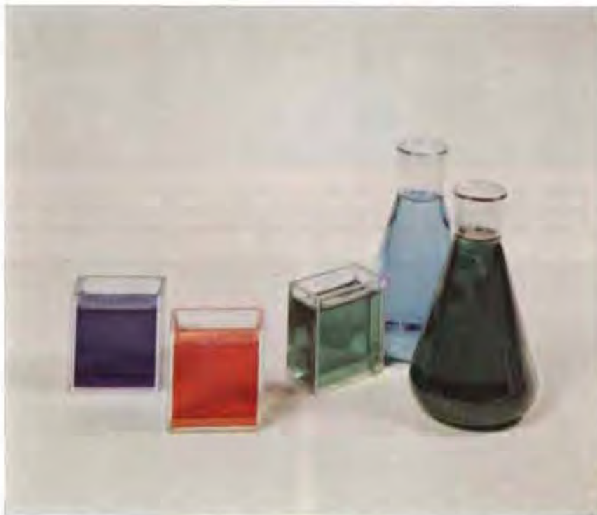
SUTTON'S FILTERS were solutions of metallic salts in glass cells. For blue he used ammoniated cupric sulfate ( far left ), for red, ferric thiocyanate ( second from left ), and for green, cupric chloride ( remaining samples ). The solutions in the cells represent the concentrations used by Sutton. The two flasks show how cupric chloride shifts to bluish-green on dilution. For transmission characteristics of Sutton's filters see top illustration on page 122.
